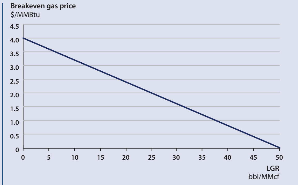
Figure 2D.3 Estimated Breakeven Gas Price ($/MMBtu) for a Mean Performing 2009 Vintage Marcellus Shale Well, with Varying Condensate Ratio (bbl/MMcf), Assuming a Liquids Price of $80/bbl
