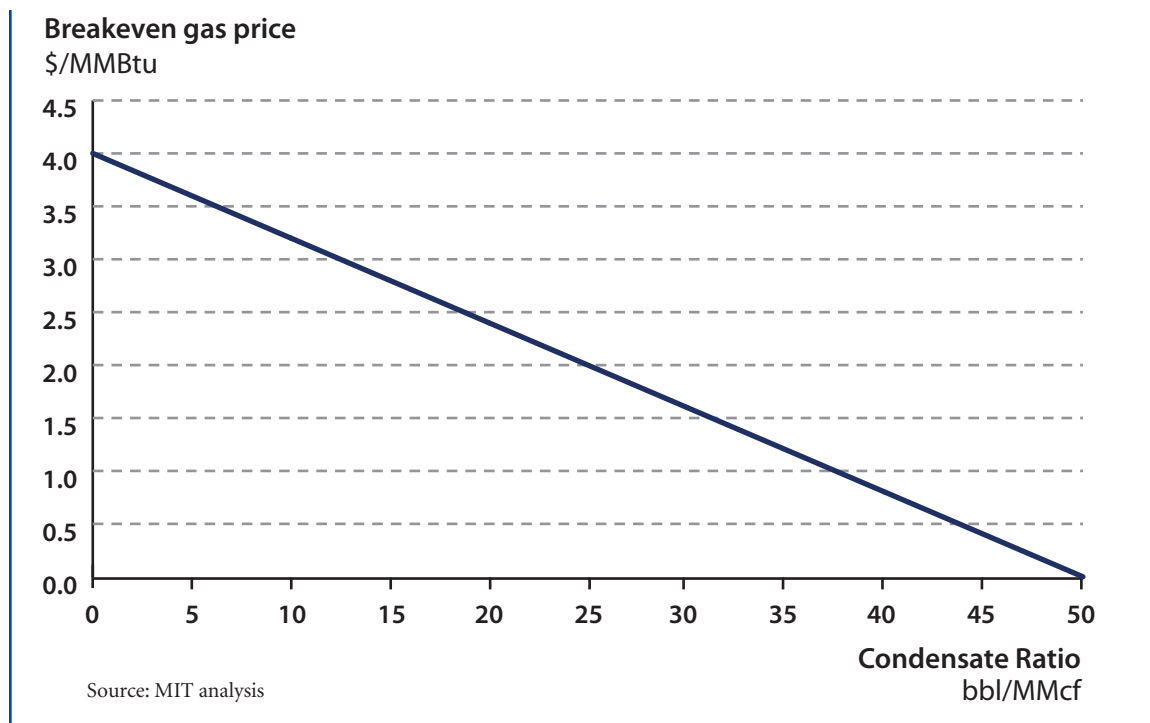
Figure 2.16 Estimated Breakeven Gas Price ($/MMBtu) for a Mean Performing 2009 Vintage Marcellus Shale Well, with Varying Condensate Ratio (bbl/MMcf), Assuming a Liquids Price of $80/bbl
